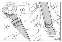
The maximum distance that the UNIBALL end fitting (A) can be unscrewed from the tie-rod body is 5 threads, or  $7.5 \ \text{mm}$  (B).
