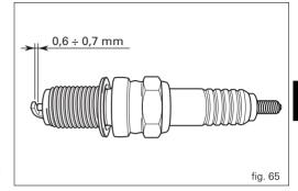
Insert the spark plug in the cylinder head and screw in fully by hand. Tighten to a torque of 20 Nm.
